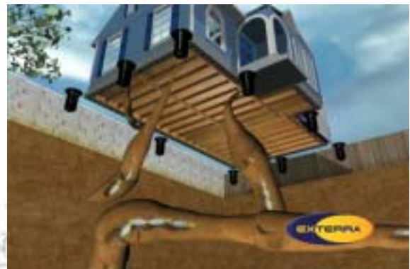
Stations Sol Exterra en place
